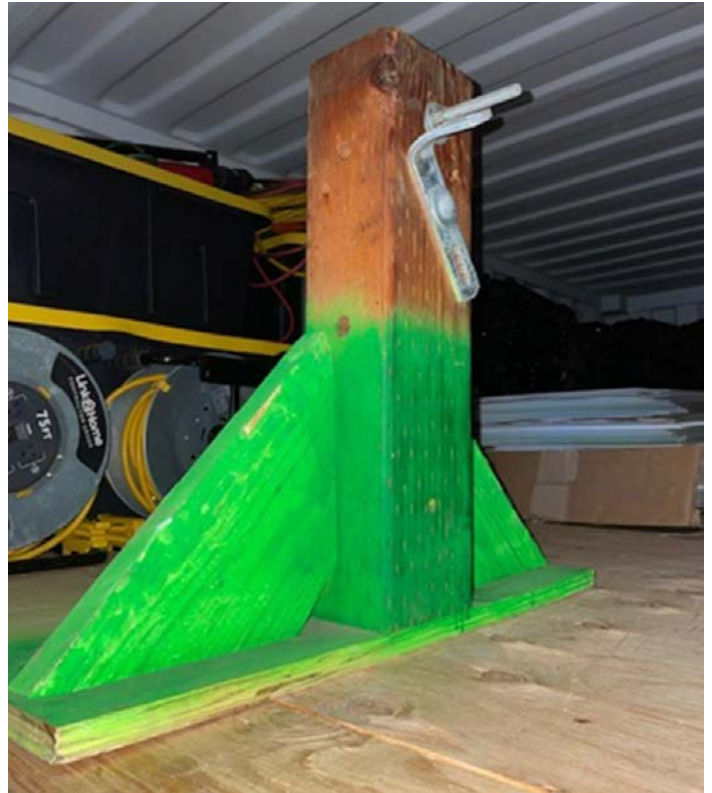
Side view of gate support
